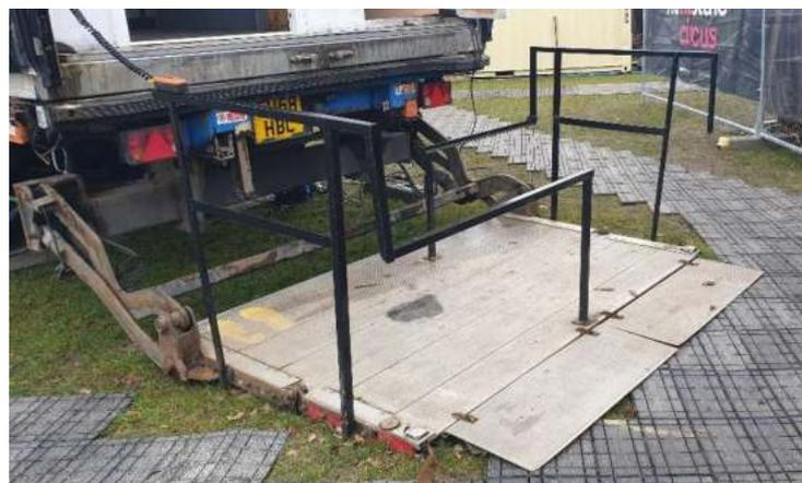
Operate the lift using the orange controller, Up and Down.
